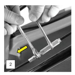
2.33 Wind the adjuster nut towards the main handlebar.
